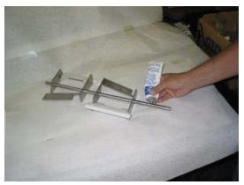
NOTICE: The black carbon ring must be facing the end of the beater bar shaft, so it will be in direct contact with the white ceramic seal inside the cylinder when the beater bar is re-installed. This is a dry seal and must be kept free of lubricants.
