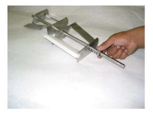
CAUTION: The beater seal may become damaged if the beater shaft is not lubricated before installation of the beater seal.
