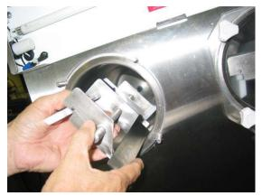
CAUTION: Do not strike the ceramic seal with the beater bar during installation!
