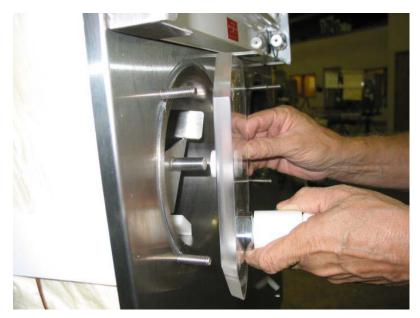
CAUTION: Do not over tighten the knobs or tighten against a beater bar that is not fully engaged in the drive plate; Permanent distortion to the faceplate may occur!
